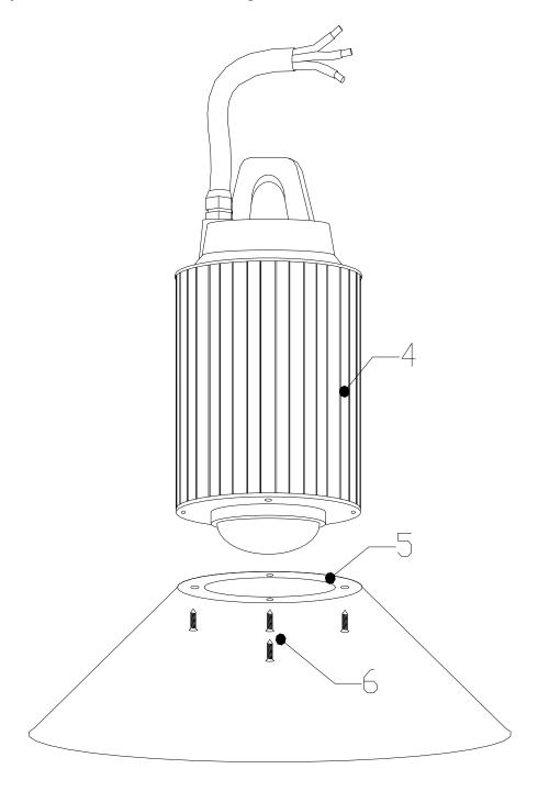
Description: 4)Lamp body 5)Reflector 6)Screws Locking screws through the Reflector on the radiator
