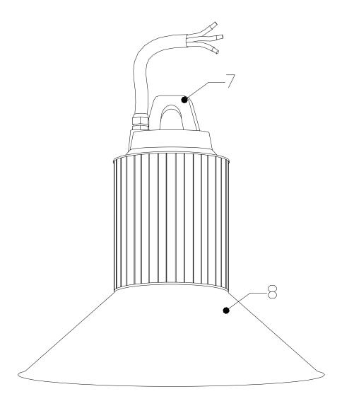
Description: 7) Hook 8)Lamp body Hook lock in the power box on the lamp body
